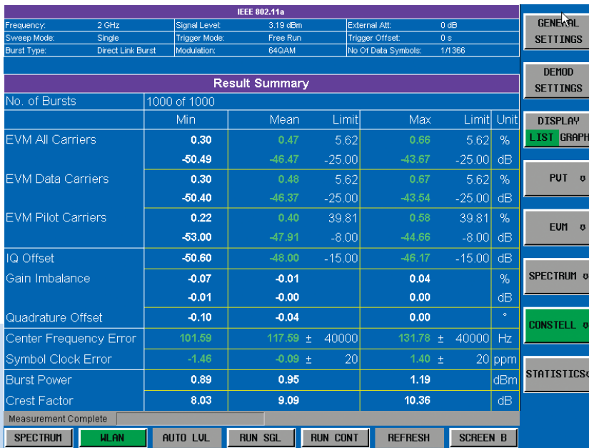
FIG 2: Display of the main modulation parameters in the Result Summary: The measurement covering 20 bursts shows an EVM of -46.7 dB for the best burst (min. peak) and -45.09 dB for the worst burst (max. peak) as well as an average EVM of -46.09 dB for all bursts. Output power (with regard to burst) and crest factor are also displayed. Quick and easy determination, for example, of the EVM dependence on the output power of an amplifier is thus possible. Owing to its auto level function, the analyzer follows these level changes without requiring any manual settings.
