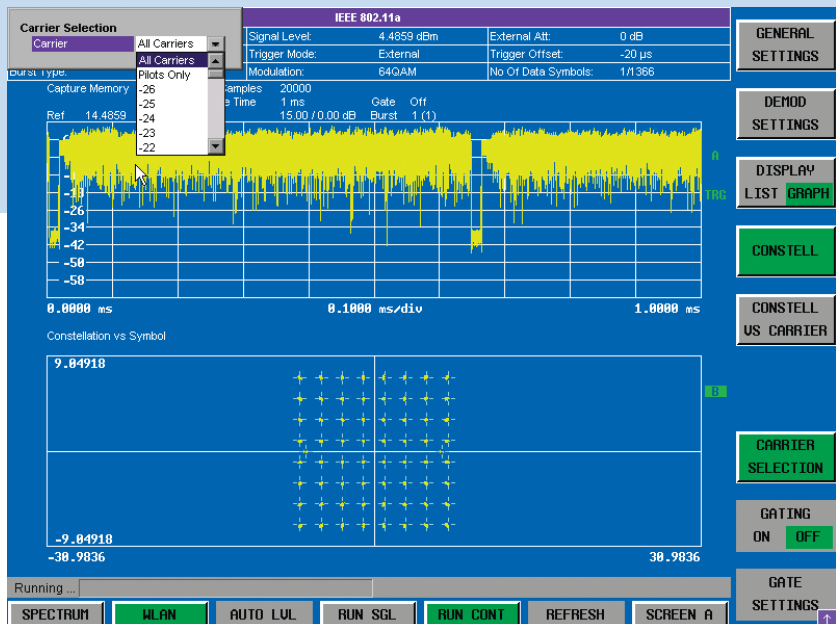
FIG 3: Constellation diagram of all or (selectable) single carriers
